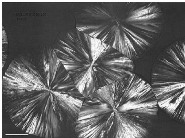
Figure 5 Polarizing optical micrograph of PTMS spherulites grown isothermally at 90°C. The bar corresponds to 50 \mu\text{m} .
